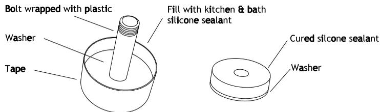
Figure 12. How to make an elastomeric compression washer.
